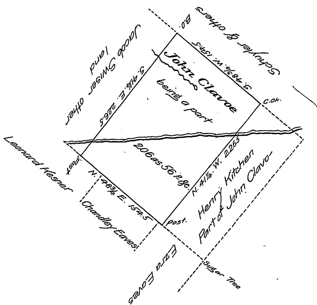
The above Survey is a part of an Original Survey made on the 10<sup>th</sup> day of June 1769 for John Clavoe on his Application dated the 3<sup>d</sup> day of April 1769 N<sup>o</sup> 1154. Situate in Madison Township Columbia County (formerly North'd) Resurveyed unto Jacob Swiser on the 27<sup>th</sup> of September 1830 Containing two hundred and Six Acres and fifty six perches & the usual Allowance
